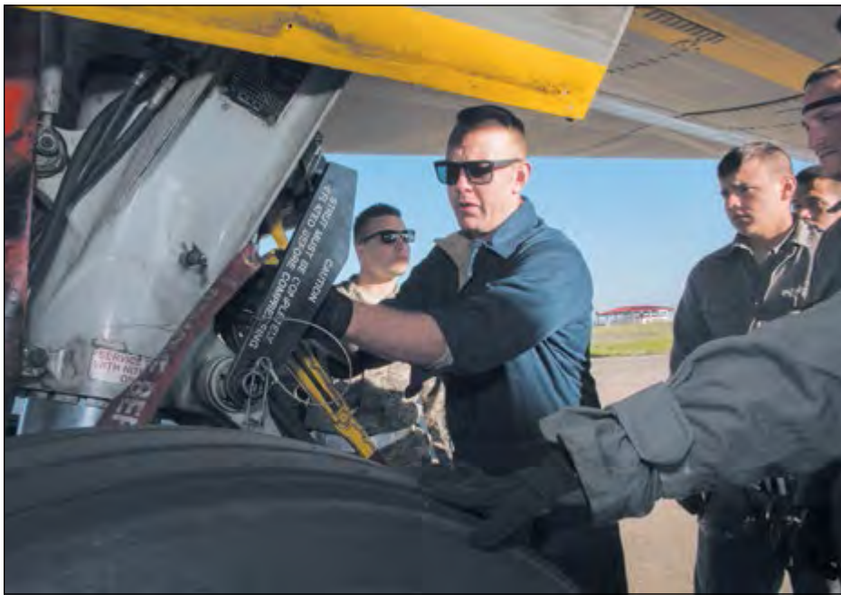
U.S. Air Force photo/Heide Couch Tech. Sgt. Adam Branam, an instructor for the 373rd Training Squadron, Detachment 14 conducts a repair demonstration for a group of crew chief trainees on a KC-10 Extender wheel assembly, Feb. 7 at Travis Air Force Base, Calif.
